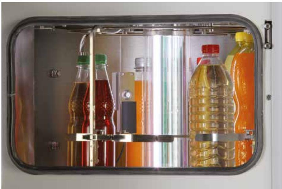
Air-cooled rotating rack test chamber including xenon lamp, optical filter lantern, and light monitor
