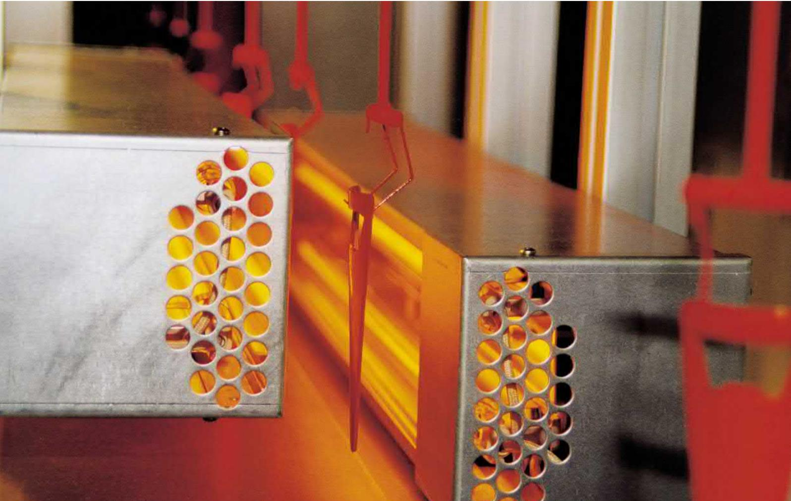
The MX module with its integrated control unit represents a system solution for the total heating process. Each module is optimised in size and wavelength to deliver energy effectively and efficiently at the surface to be heated.
