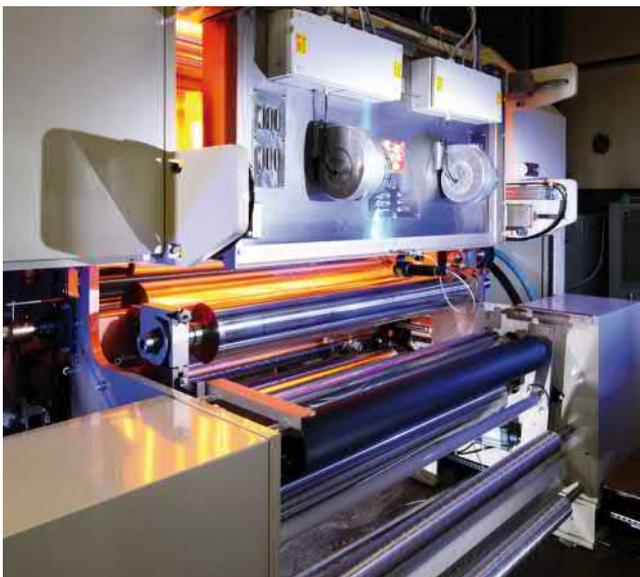
Plastics require very exact temperature profiles during production to achieve their high quality look. These temperature profiles are provided by MX infrared modules.
