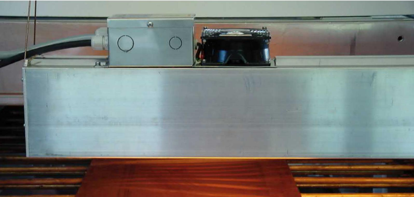
Simply Constructed Modules contain one or more infrared emitters. They can be easily retrofitted into existing production plants and because of their long operation lives, they are extremely cost-efficient.
