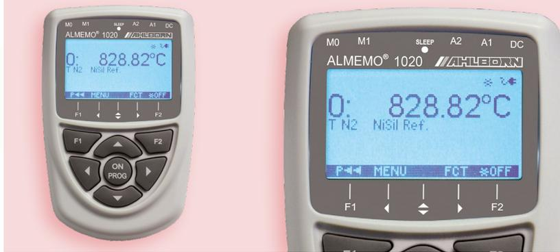
**Reference measuring instrument for temperature**
