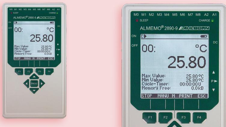
**ALMEMO® precision measuring instrument with data logger function. Comprehensive range of functions for all application areas. Increased measuring accuracy, fast measuring rate. Generously dimensioned graphics display, bright illumination. 9 measuring inputs Runs on rechargeable batteries, charging via the device itself**
