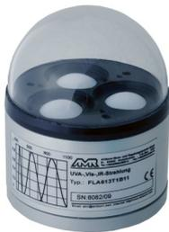
Probe for measuring global radiation FLA 613 T1B11,
