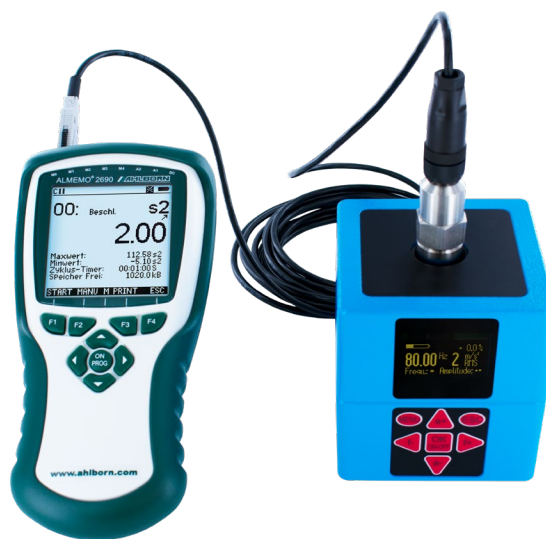
ALMEMO® measuring device with vibration sensor FSA 084, mounted on the vibration simulator
