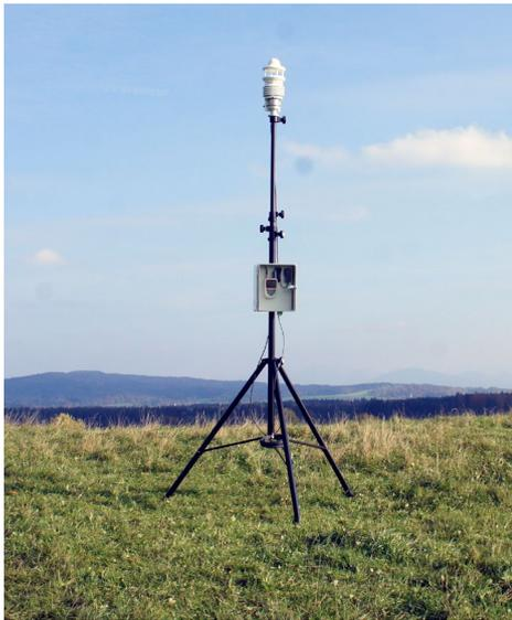
Professional weather station for mobile use to measure all relevant meteorological parameters. Quick and easy to install, robust design, compatible with various ALMEMO® V7 data loggers.
