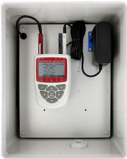
**Weather-proof housing AG2 for ALMEMO® 202-S / 204 and meteorological sensor**
